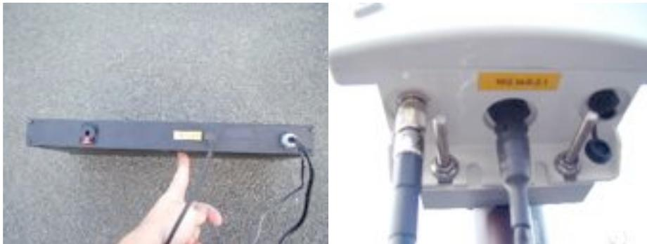
Left: Encoder unit, shown out of rack. Note ethernet cable plugged into jack. Right: Transmitter / Receiver. Note Rotary ethernet cable attached in the middle.
