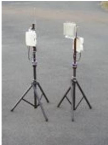
Photo: Omnidirectional Link Kit (left) and Directional Link Kit (right)
