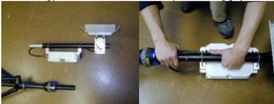
Finally take the provided outdoor Ethernet cable (dark grey, standard ethernet jack on one end, rotary connector on the other end), and plug it into the standard Ethernet jack on the back of the Encoder unit in the Output Pack Control Rack. Then take the other end of the cable, and carefully attach it to the jack on the bottom of the white transmitter / receiver unit. Note that you plug the cable into the jack, and then rotate the locking collar to hold it permanently in place.
